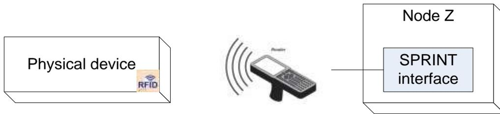
Figure 6-7: Registration of physical device using RFIDs
